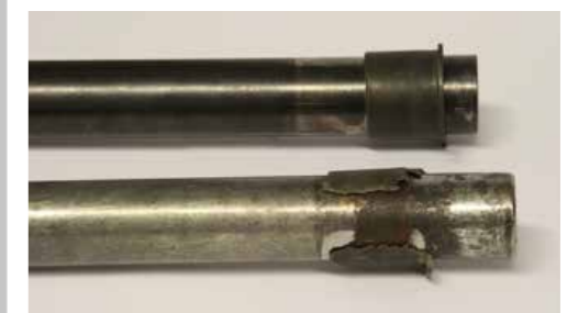
Top: galvanised pin, bottom: the nitrocarburised pin (Source: igus® GmbH).
