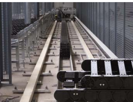
The P4.32 e.chain® supplies energy to a pallet truck in tobacco production.
