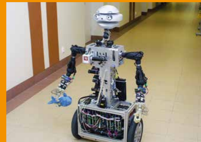
The Technical University at Wroclaw, Poland equipped its autonomous robot FLASH with 2 robotlink® articulated arms, each with 4 DOF.
