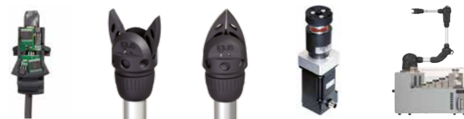
Angle sensors ► Page 15 2-jaw gripper ► From page 18 3-jaw gripper ► From page 18 Drive units ► From page 20 Complete 6 DOF unit ► From page 24
