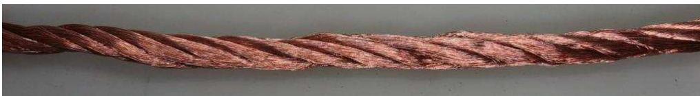
The copper conductor.
