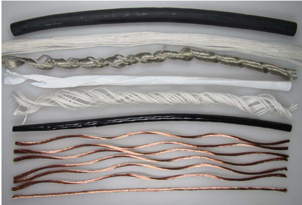
Overview of the dissected pieces of the cable no.1.2, point of the fixed point after 17.099.049 cycles.
