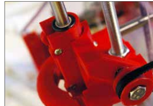
Accurate printing of 3D plastic models: drylin® linear guides and iglidur® plain bearings in use at high speeds
