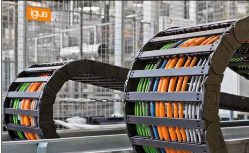
Cable service life test at the igus® lab, Cologne
