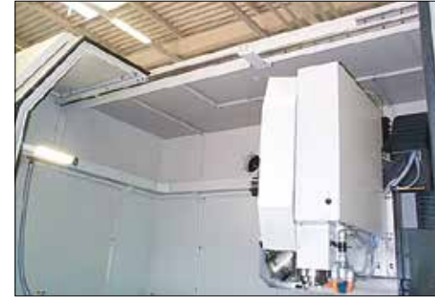
Machine doors with maintenance free guide using drylin® linear technology.
