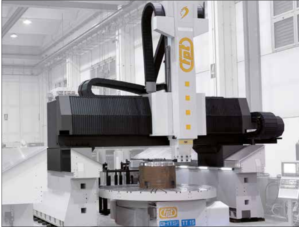
A wide range of e-chains® in a CNC machine tool – hanging, upright, rotated, and unsupported.
