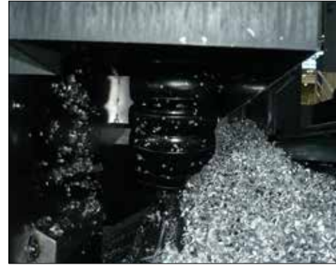
igus® RX e-tube - ideal in the direct chip area, IP protection class 40
