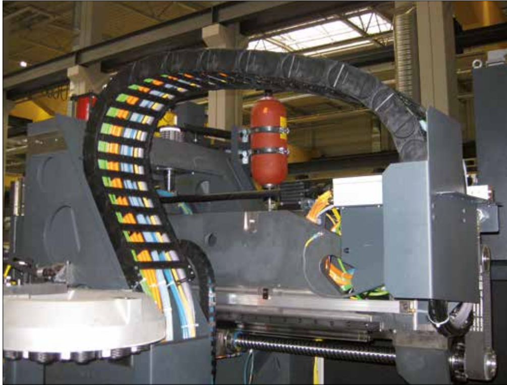
Sliding column machine: to keep installation space and costs for the e-chainsystem® very low, an igus® E4.42 Series was installed upright with single-sided radius in the travel.
