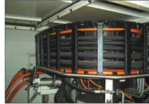
e-chain® E6 in a CNC grinder: The low weight supports particularly smooth motions.
