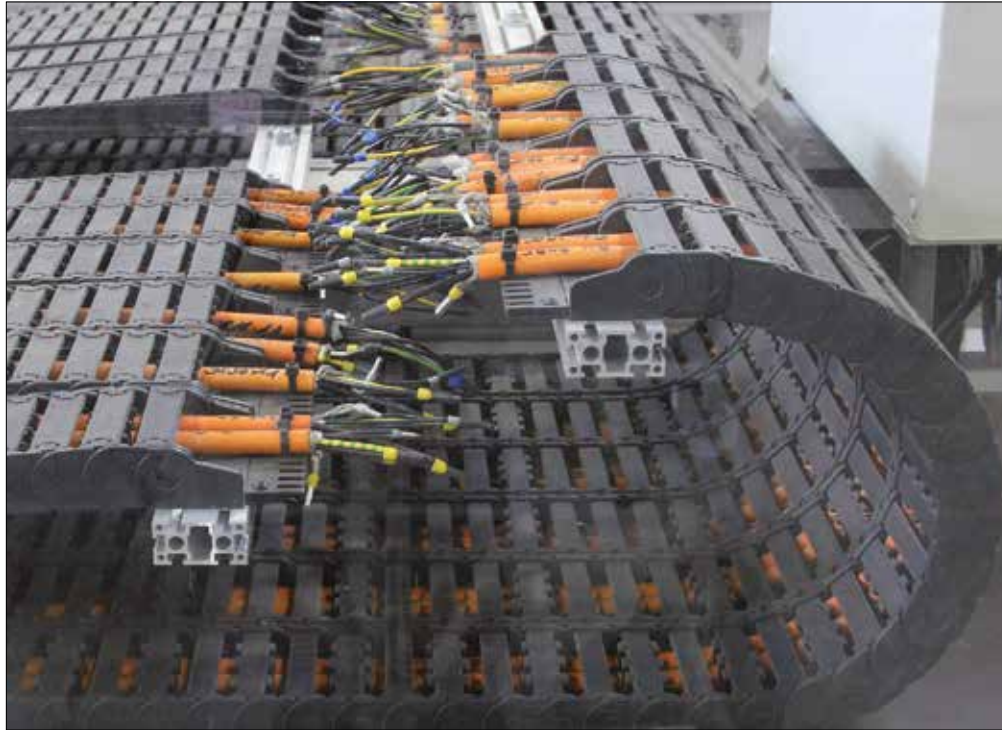
Cable service life test at the igus® lab, Cologne
