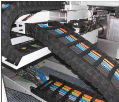
Combined motion with an igus® E6 readychain®.
