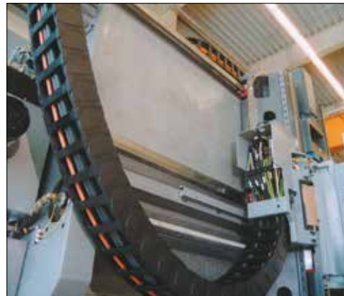
The e-chain® can also be supplied without camber if space is limited.
