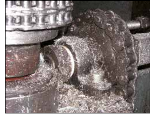
Dry-running igubal® plastic spherical bearings - no chip adhesion
