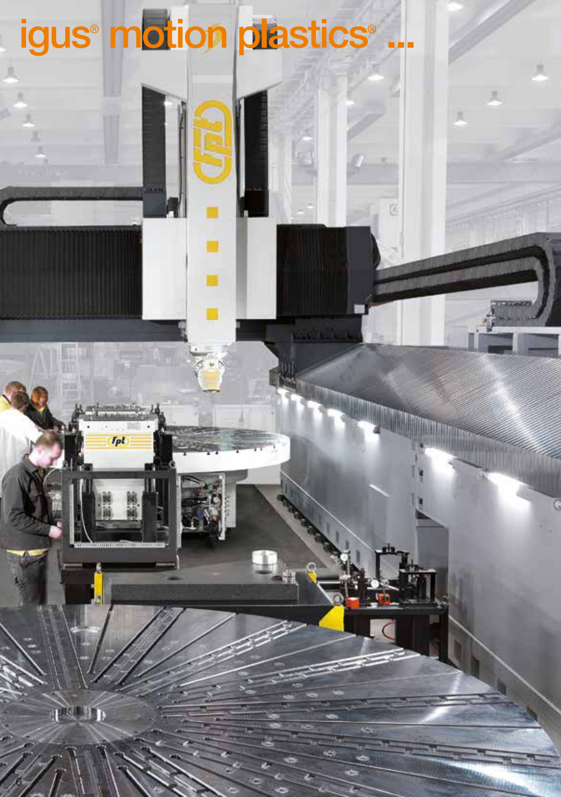
igus® RX e-tube - ideal in the direct chip area, IP protection class 40
