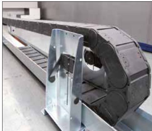
Horizontal guidelok upper run guide for long travels in chip areas.
