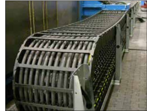
For long travels in the chip area - guidelok horizontal guides up to 50 m
