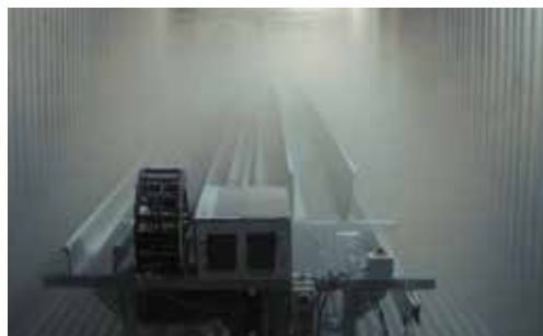
Cold tests on cables and energy chains at -40°C
