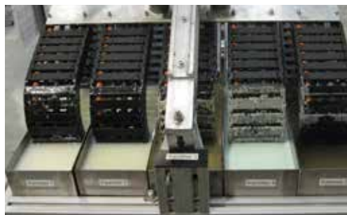
Media tests: test of the durability in adverse chemical effects in motion
