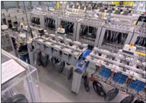
Tribological tests in the plain bearings laboratory, igus® Cologne.
