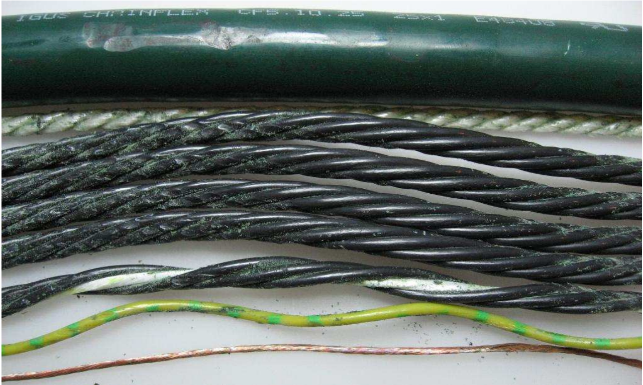
Overview of the dissected pieces of cable of no. 1.2 CF5.10.25 after 41.538.456 strokes
