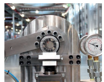
Heavy-duty test rig for plain bearings
