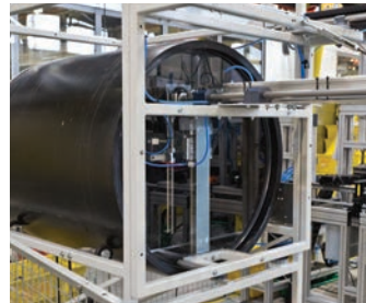
Tightness testing on e-tubes
