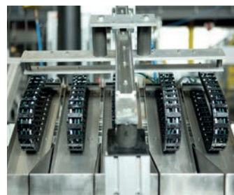
Oil-resistance testing on cables
