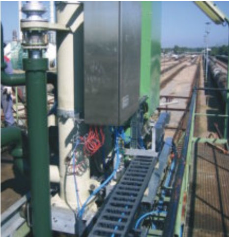
igus® ESD option of the system E2/000 in a tank car filling station. 100% ATEX safety must be ensured during the transport of gases.
