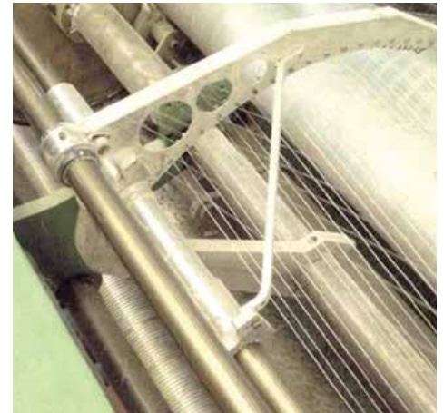
Lubricant-free: DryLin® R in weaving machine Schmierfrei: DryLin® R in Webmaschine
