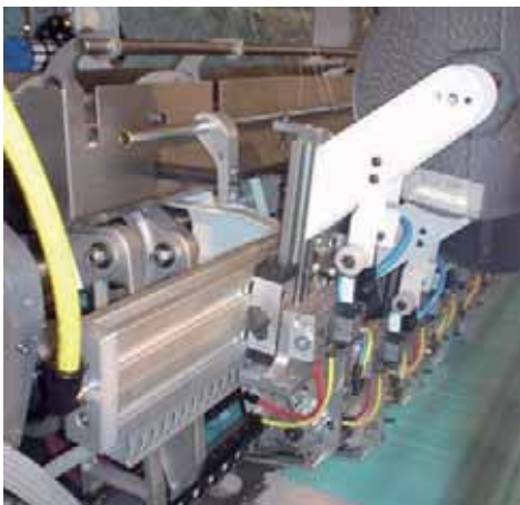
Wear resistant: DryLin® T in quilting machine Verschleißfest: DryLin® T in Steppmaschine
