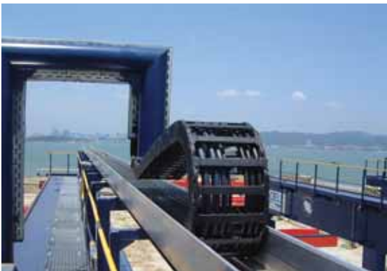
Crane builder Noell in Panama. Application: RTG; Travel: 19,5 m; speed 60 m/min.
