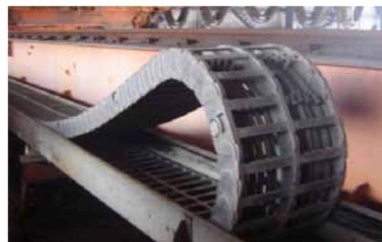
Heavy Duty E-Chain® in indoor crane in steel plant in India
