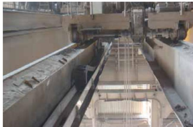
Even in dusty environments: E-Chain® trough in slack yard crane
