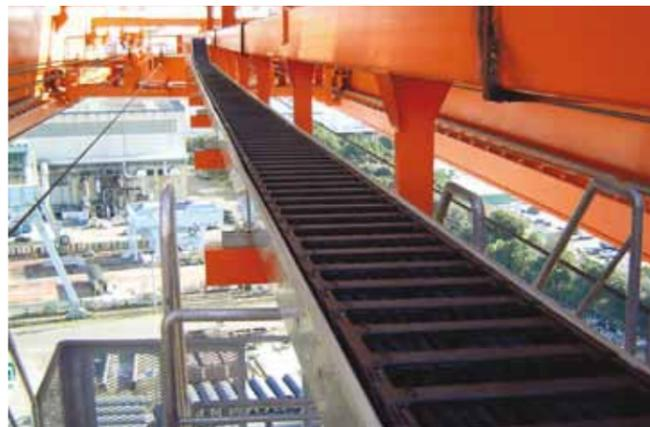
Long travel with igus® steel guide troughs and a harnessed E-Chain® in a crane application
