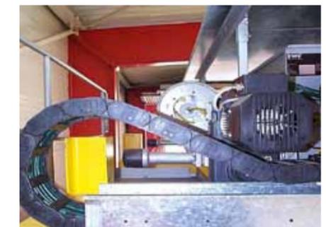
The cranebeam's end is also the end of the E-Chain®
