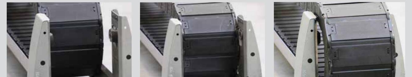
The E-Chain® is guided in the trough channel, pushing back the spring loaded roller support with its radius...
